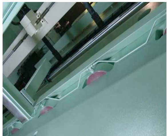
油壓式撓曲補償系統 Hydraulic Crowning Compensation System
